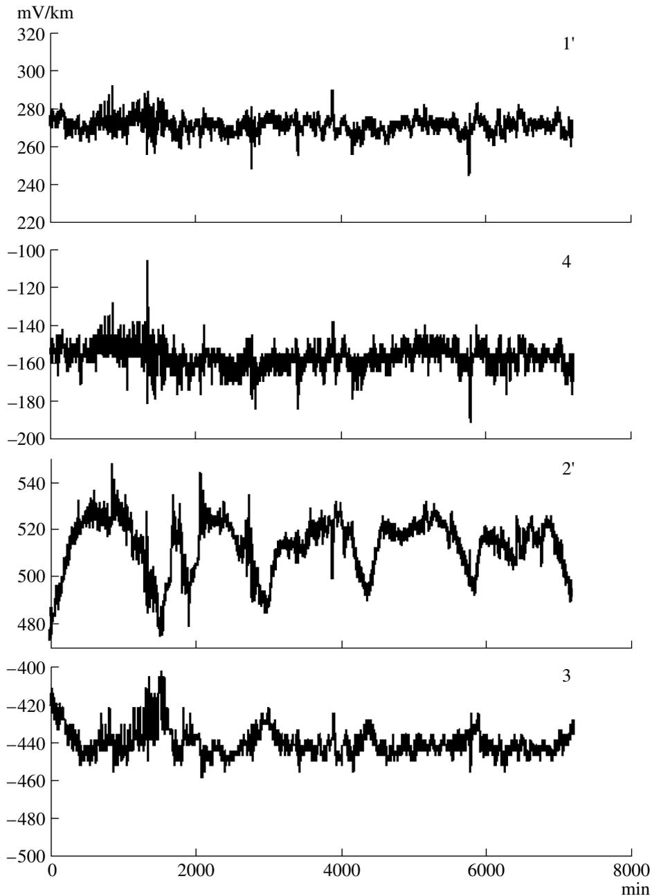
**Fig. 5.** Comparing the plots of electrotelluric field intensity. Numerals 1' and 2' denote the plots obtained by rotating the axes 1 and 2 by an angle of  $40^\circ$  in the counterclockwise direction, i.e., until they coincide with lines 3 and 4 (see Fig. 3).
