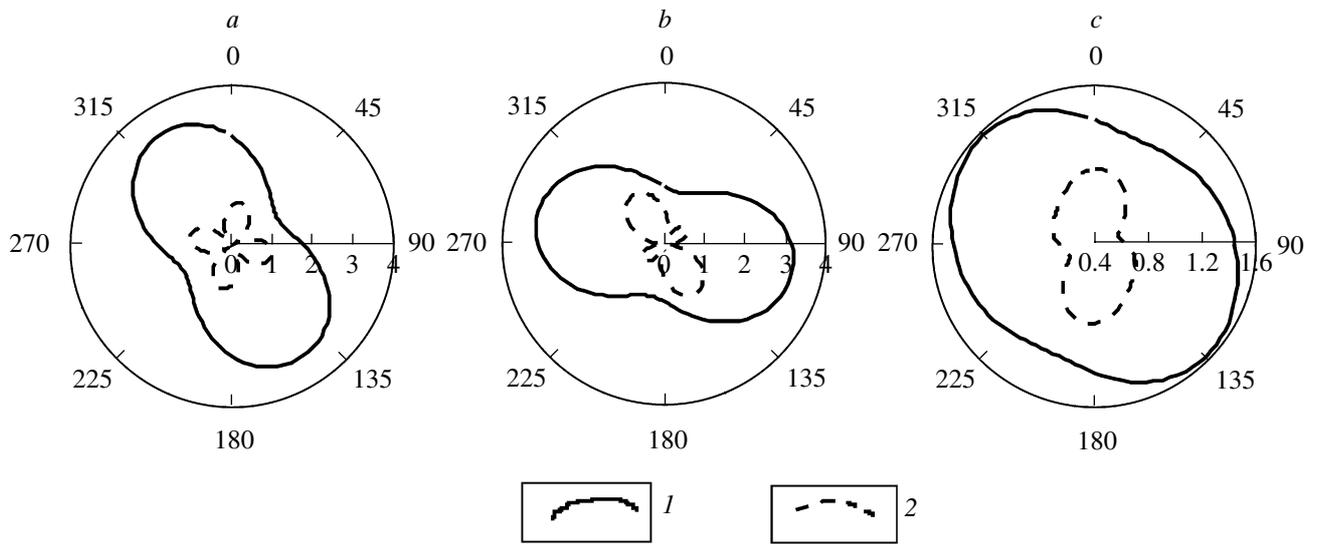
**Fig. 8.** Polar impedance diagrams. *a*, *b*, and *c* are for lines 1, 2; 4, 3; and 1', 2', respectively: (1) diagrams of the principal and (2) diagonal impedance.
