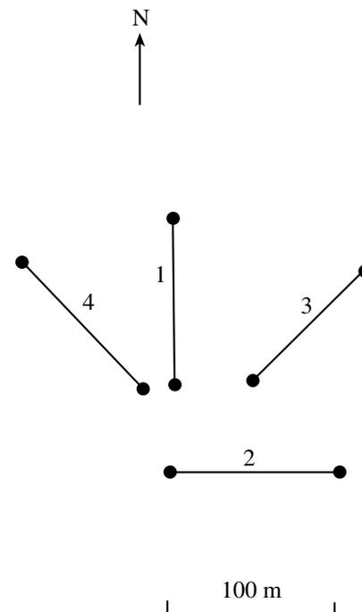
**Fig. 3.** A map showing the positions of measuring lines at the Tundrovyi site. 1, 2, 3, 4 are identification numbers of receiving lines. Azimuths of lines: 1 – 0°; 2 – 90°; 3 – 40°; 4 – 310°. The scale is shown for the measuring lines.
