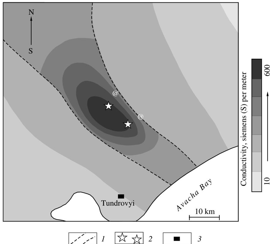
**Fig. 2.** A map of total conductivity in the volcanogenic sedimentary cover in the area of study: (1) lines of equal conductivity, (2) volcanoes, (3) Tundrovyi station.
