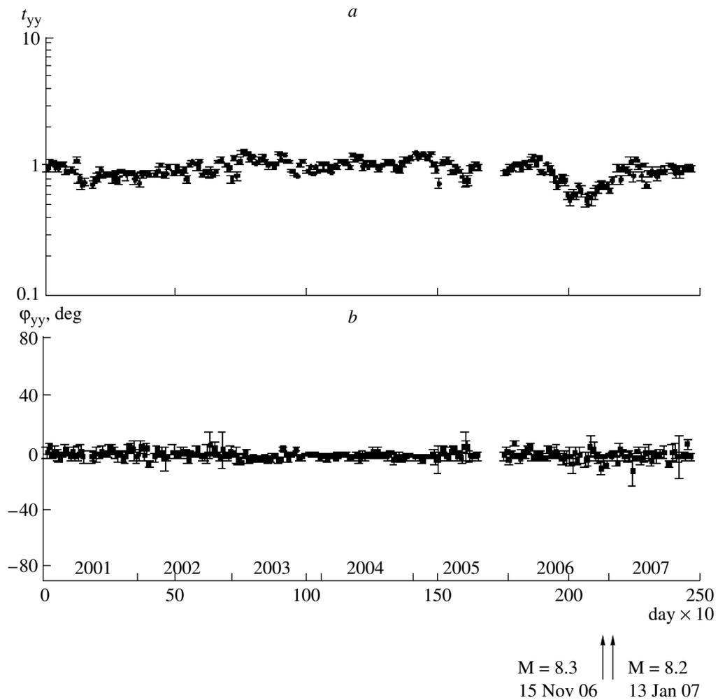
**Fig. 9.** Plots of the absolute value of the telluric tensor component  $t_{yy}$  (*a*) and its argument  $\phi_{yy}$  (*b*). The dates of great earthquakes ( $M = 8.3$  and  $8.2$ ) occurring in the Kuril–Kamchatka island arc area during the past 30 years are marked on the time axis.
