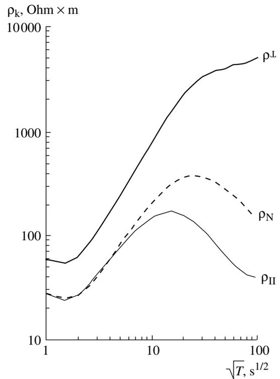
**Fig. 7.** Modeled MTS curves.  $\rho^L$ ,  $\rho^{\perp}$ , and  $\rho_N$  are the MTS longitudinal, transverse, and locally normal curves.
